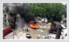
A scene from the recent LASTFIRE testing program aimed at assessing the performance of new foam formulations – Fluorine Free and C6 fluorosurfactant based – for bund spill fire application.
